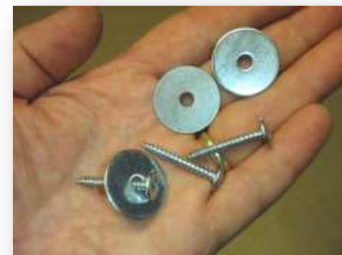
Fender washers and lath screws for attaching exclusionary mesh
