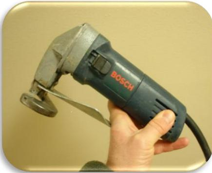
When using welded-wire mesh, renting a metal-cutting shears can help considerably if you are cutting lots of mesh for a big job, such as a very large deck
